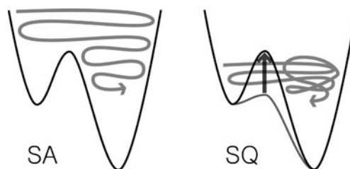
Fig. 6 Schematic diagram illustrating conformational searching performed by SA and SQ. In SA, conformations are sampled as the system energy is lowered according to the cooling scheme, as represented by the gray line on the left figure. On the contrary, conformational searching during SQ is done with small energy variations and with the changing barrier height according to the variations of q parameters, as illustrated in the right figure
